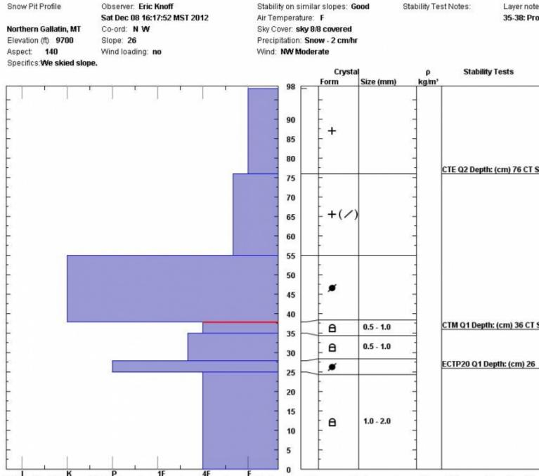
I K P 1F 4F F U Notes: The stability on similar slopes is good as long as the slope angle is less than 35 degrees. On steeper slopes with a similar aspect and elevatior stability is fair.
