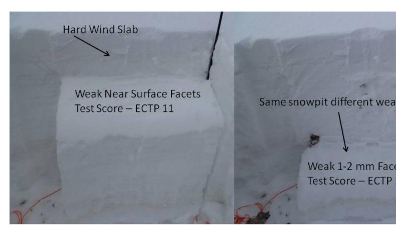
Weak layers near the surface and near the ground are producing unstable test results in Middle Basin. Photo: GNFAC
