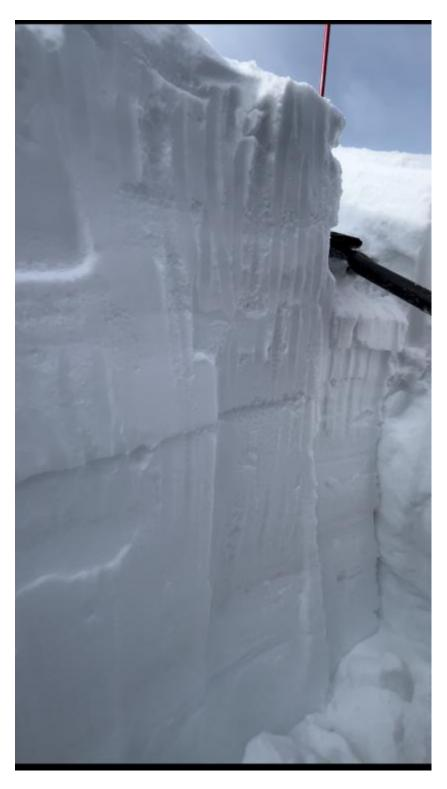
We got an ECTP18 result on a north aspect at 8600' in the absarokas. It propagated on a small layer of facets 30cm down. Photo: C von Avis
