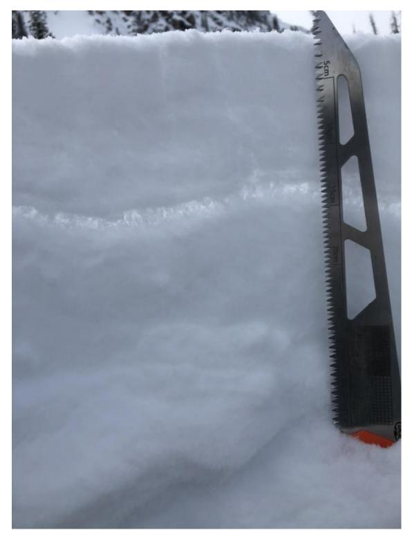
From obs: "Observed large surface hoar grains preserved 10 - 25cm below the new snow surface. Photo taken in the flats of goose creek outlines most prominent weak layer in the pack. I suspect these grains are larger than most because of increased sun exposure in the valley bottom during the dryspell. Pits on north facing aspects didn't show such a pronounced weak layer but evidence still exists of buried surface hoar layer." Photo: J. Wenzel
